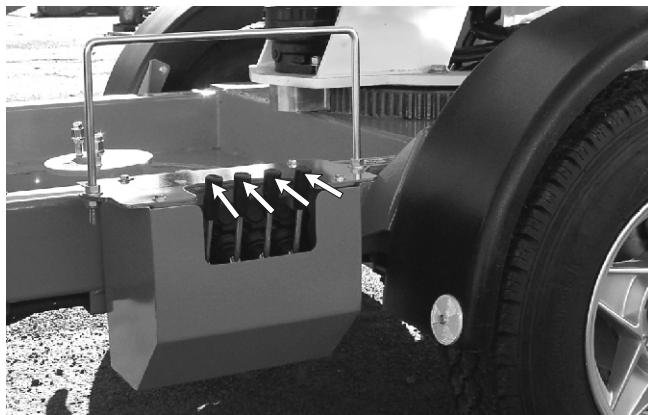
Figure 6.9 - Stabiliser Controls (Manual)
