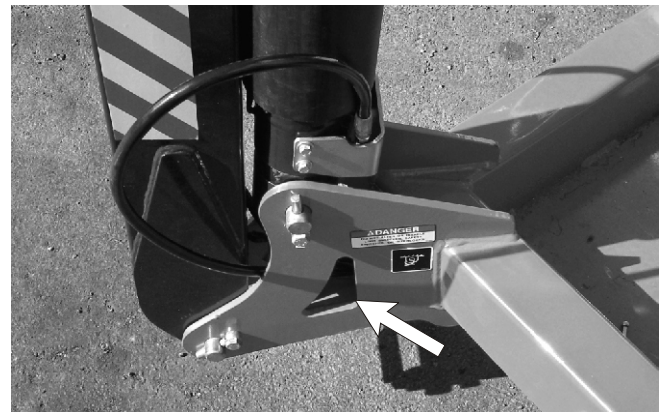
Figure 10.4 - Tie Down Lugs
