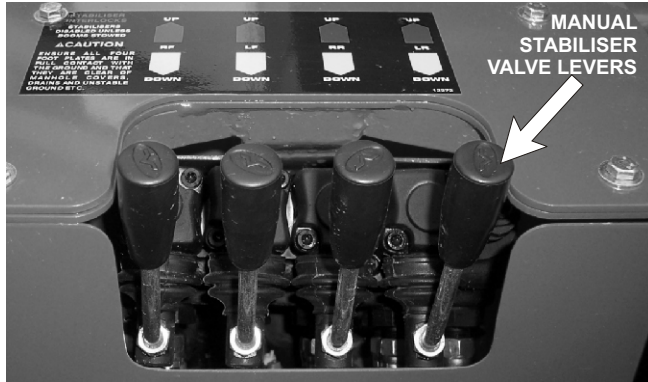
Figure 6.7 - Stabiliser Controls (Manual)
